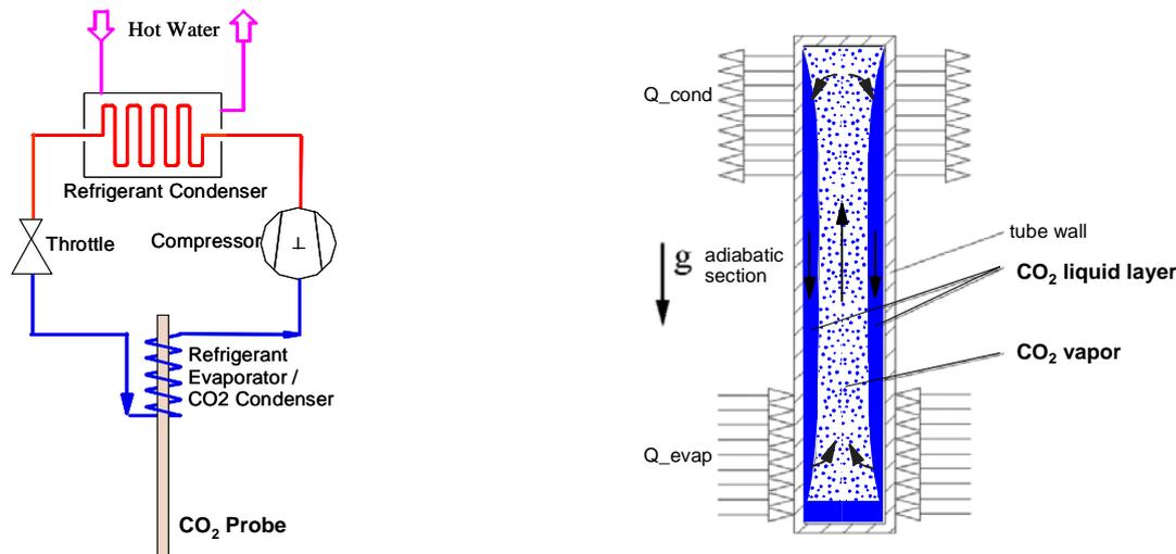
Figure 10: System layout (left) and working principle of a CO<sub>2</sub> probe, i.e. closed two-phase thermosiphon (right)
