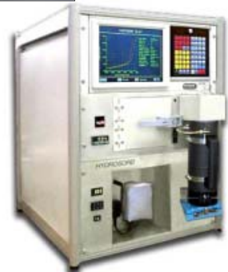
Automatic water-vapor adsorption measurement apparatus
